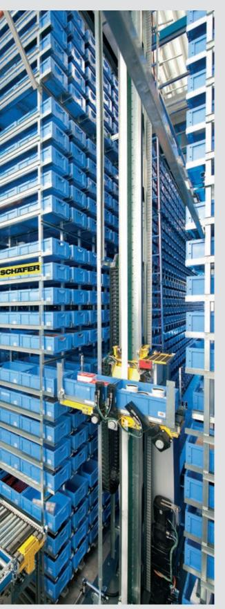
With the Schaefer Miniload Crane (SMC), SSI SCHAEFER completely covers rack automation for totes, cartons, and trays and presents the ideal solution for maximum use of vertical storage while using very little floor space.
